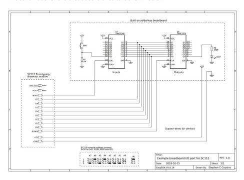
Address decoding is set to write to the output port when the processor writes to I/O address 0x50 or 0x51, and read from the input port when the processor reads from I/O address 0x50 or 0x51.
