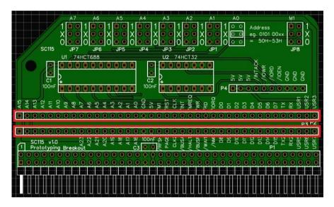
P3 is only required for signals on the enhanced bus (the second row), so it may not be necessary to fit this connector.
