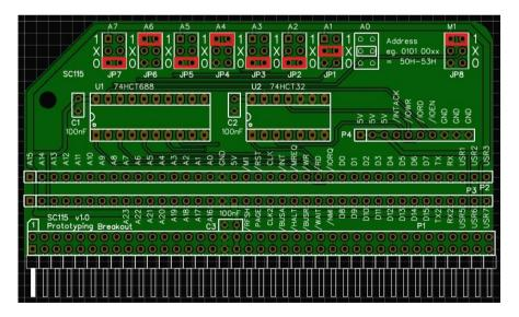
This works as 50 hexadecimal to 53 hexadecimal is 0101 0000 binary to 0101 0011 binary. When the "don't care" bits are substituted, it is 0101 00XX.
