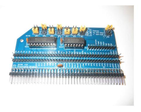
The module includes address decoding adequate for most I/O devices, thus saving the need to build a decoding circuit for every prototype. Address decoding is very flexible, allowing a configurable start address and a configurable range size.
