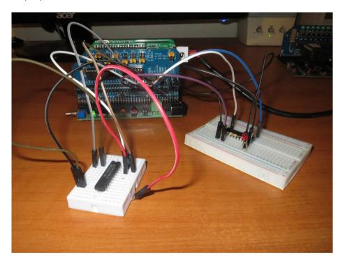
The breakout module provides access to all the necessary signals which are connected to solderless breadboards with Dupont cables.
