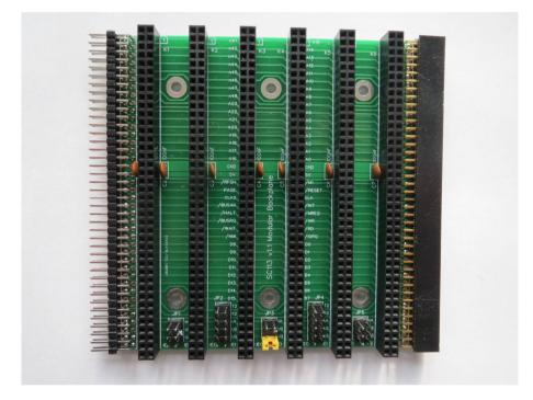
Pin 40 of the standard RC2014 bus is used for the Z80 interrupt daisy chain signal IEO, with the 40<sup>th</sup> pin of the enhanced bus, sometimes called pin 80, being used for the IEI signal. These two pins therefore do not connect to all 6 sockets in parallel, but instead link pin 40 of one socket to pin 80 of the next, forming a chain.
