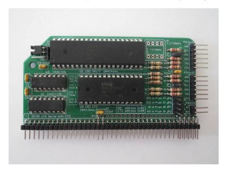
Each port has transmit, receive, request to send and clear to send signals brought out to connectors on the back edge of the module. The transmit and receive signals can be connected to the appropriate RC2014 bus pins.
