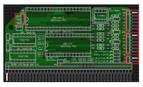
P2, P3 and P4 can be fitted as a single strip but with two pins pulled out at the gaps between P2/P3 and P3/P4.
