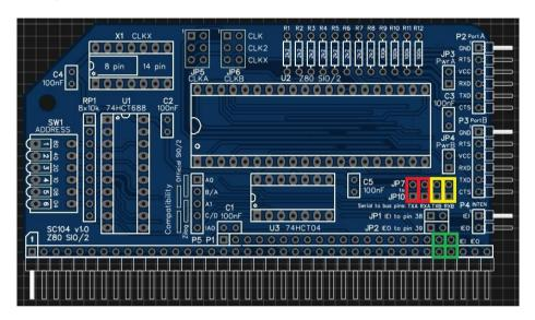
The jumpers highlighted in red are for serial port A and those in yellow are for serial port B. The pins used on the RC2014 bus are shown in green.
