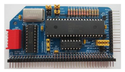
Each port has transmit, receive, request to send and clear to send signals brought out to connectors on the back edge of the module. The transmit and receive signals may also be connected to the standard RC2014 bus pins via jumpers.
