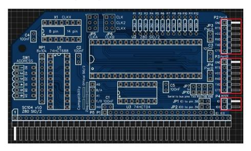
P2, P3 and P4 can be fitted as a single strip but with two pins pulled out at the gaps between P2/P3 and P3/P4. The photograph at the beginning of this guide shows the board assembled with the connectors in a single strip.
