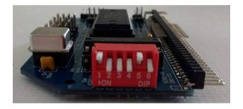
In order to be compatible with existing RC2014 software the first SIO module needs the base address 0x80, with the module occupying I/O address range 0x80 to 0x83.
