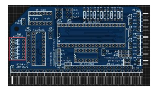
In order to provide some certainty for software it is strongly recommended you set the base address of your first SIO module to 0x80. The module then occupies I/O addresses 0x80 to 0x83. This is done by setting the switches as illustrated below.
