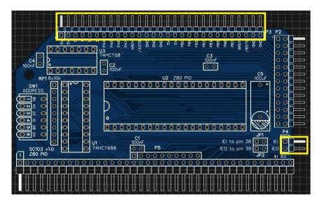
Connector P3 is optional, so if you want to put the RC2014 in a case or just don't like the look of it, you can leave this connector off. Alternatively you might prefer a different connector, such as a female header socket.
