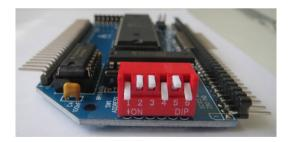
If you have a second PIO module the recommended base address is 0x6C.
