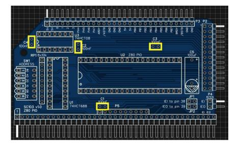
Fit and solder resistor pack RP1.
