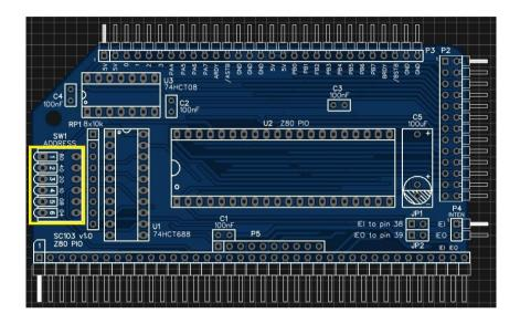
In order to provide some certainty for software it is strongly recommended you set the base address of your first PIO module to 0x68. The module then occupies I/O addresses 0x68 to 0x6B. This is done by setting the switches as illustrated below.
