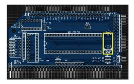
The PCB allows for a radial or axial capacitor. In order to build a low profile board, the capacitor should lay on its side. An axial capacitor would be most secure in this configuration, but there is limited length allocated and you probably don't have one!
