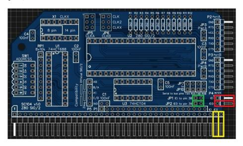
Note that v1.0 of the PCB has the IEI and IEO bus pins incorrectly labelled. It indicates the use of pins 37 and 38, not 38 and 39.
